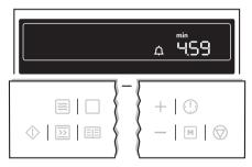
When the time set has elapsed, an acoustic signal sounds for 2 minutes. "0.00" lights up and the symbol for Countdown [4] flashes.
